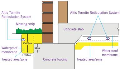
The two products are the 150mm wide perforated sheet with one dripper line and the 300mm unperforated sheet also with one dripper line. These two products can be used singularly or in combination.
